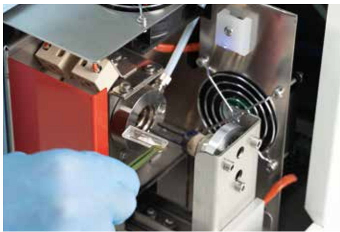
Boat with sample is placed inside the system
